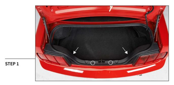
Use a flat-head screwdriver to remove the 4 clips holding the plastic trunk trim in place.
