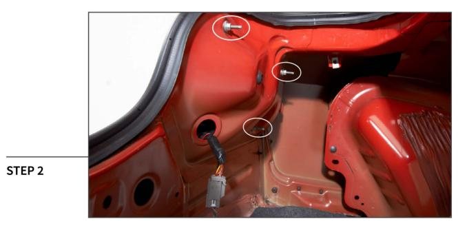
Unplug the wiring harness and use an 11mm socket or wrench to remove the 3 nuts holding securing the tail lights. Push out the rubber grommet, where the harness feeds through the sheet metal, and remove the light.
