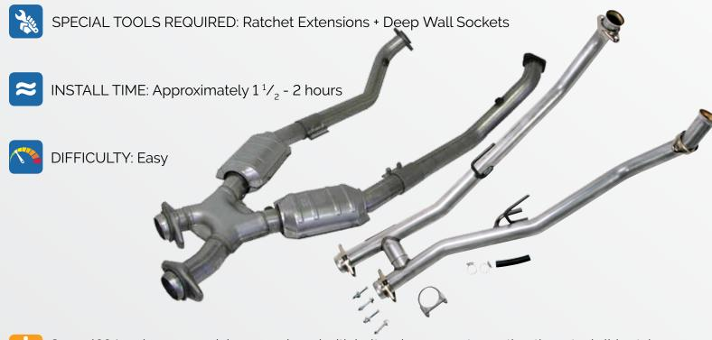
Some 1994 and newer models are equipped with bolt on hanger system rather than steel slide style used on the 1986-1993 models. To remove simply unbolt the H-Pipe from the hanger mount.
