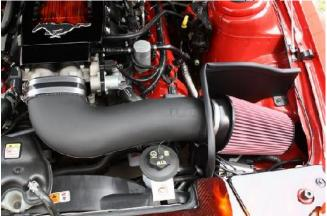
Plug in MAF sensor and supplied PCV hose (hose can be shortened to your liking depending on how you route it) Use light oil to help slide hose onto fitting in the bottom of the tube.
