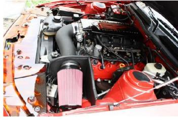
This kit includes an S&B Powerstack pre-oiled reusable air filter. The frequency you should clean your filter will depend on your driving conditions. It is recommended to check your filter at every oil change or 3,000 miles. If there is a build up of dirt as thick as the wire mesh, then it's time to clean your filter. As dirt builds up on your filter, the restriction of the airflow also increases. More frequent cleanings will improve your fuel economy and your vehicle's performance.
