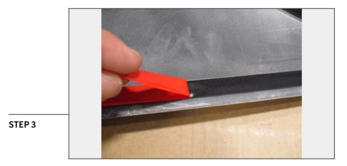
Peel backing from adhesive tape on the side scoop.
