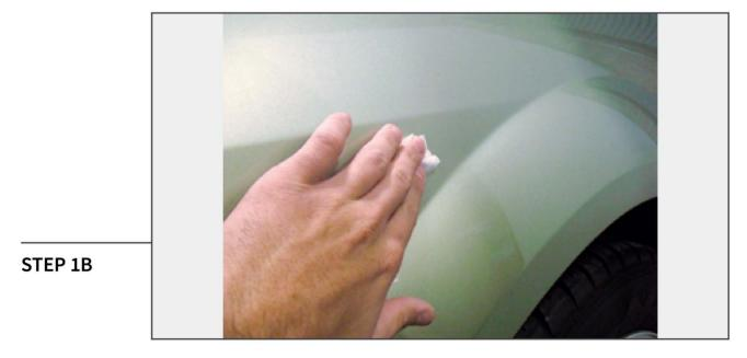
Using the supplied Alcohol Prep Pads, thoroughly clean the surface of the vehicle where the scoop will be applied. Once dry, treat the same area with the supplied adhesion promoter.
