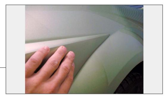
When certain that scoop is properly aligned, press down firmly where adhesive tape was applied to ensure a proper fit.
