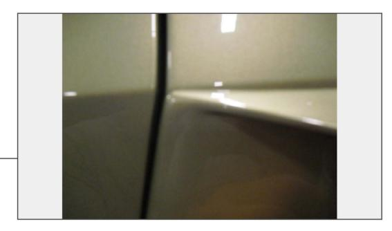
Lightly place side scoop on vehicle, taking care to align upper corner with body line and door opening as shown below.
