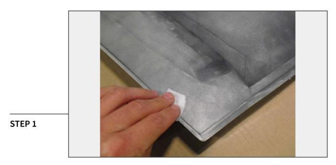
Using the supplied 3M Automotive Adhesion Promoter, thoroughly clean the surface of the side scoop where the adhesive tape will be applied.
