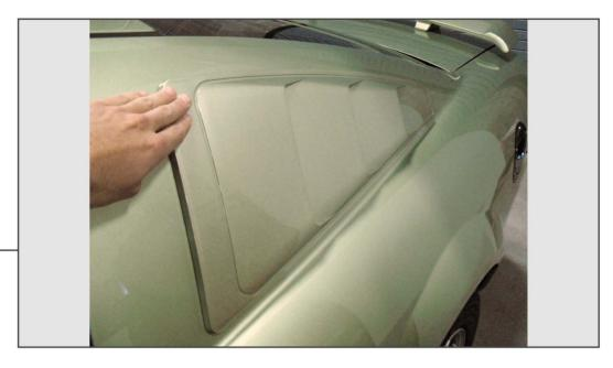
Once louver is in desired location, firmly press down on all surfaces where adhesive was applied to ensure a proper fit. Repeat all steps for remaining louver to complete installation.
