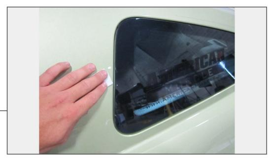
Using the supplied Alcohol Prep Pads, thoroughly clean the area around the rear quarter windows where the scoops will be placed.
