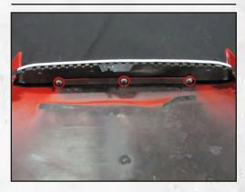
Install the honeycomb insert into the scoop and secure it with the 3 provided locking rings.
