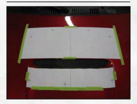
Install the lower template first by lining it up on the edge of the factory insert and along the two outside edges as shown. The upper template is installed on the upper edge of the factory insert, using the dotted center line as a guide (this dotted line should be matched with the dotted line on the lower template). The photo below shows both templates properly installed on the hood.
