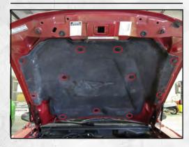
Open the hood and remove the 11 plastic retaining pins securing the hood insulation pad. A trim removal tool works best for this job, but a flat head screwdriver can be used. Once all of the clips are removed, set the insulation pad aside.
