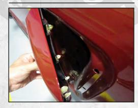
Install the new side scoop by locating the forward retaining clips in the body holes as shown, followed by the rear. Once all clips are loosely installed in the body holes, press down firmly to fully seat the clips in the body.
