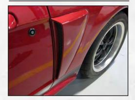
Repeat Steps 1-5 for opposite side scoop to complete the installation. If for any reason you ever need to remove the scoops, repeat Step 1 using a plastic trim removal tool to release the plastic retaining clips.
