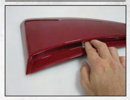
Using the supplied alcohol pad, thoroughly wipe the area where the honeycomb insert will be applied.
