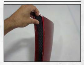
Peel the backing from the 3M adhesive tape on the insert and place it inside the opening of the scoop. Place the bottom of the insert in first, working your way to the top. Once properly aligned, press down firmly to fully seat the adhesive tape.
