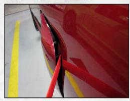
Remove the factory side scoop by carefully inserting a plastic trim removal tool and prying the retaining clips off. Start at the rear of the scoop, finishing with the front edge.
