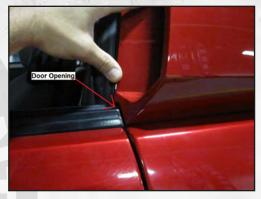
Then, line up the front edge of the louver with the door opening molding. Once the louver is in the proper position, press down firmly to fully seat the adhesive tape.
