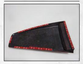
Let the Adhesion Promoter set up for 30-60 seconds, then apply the adhesive tape as shown.
