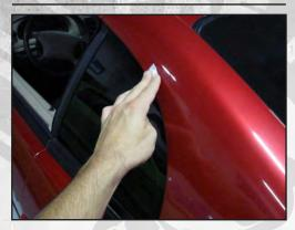
Thoroughly wipe the area of the quarter window where the louver will attach with the supplied alcohol pad.
