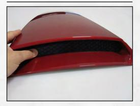
Peel the backing from the adhesive tape and place the insert into the louver opening as shown. Once properly aligned, press down firmly to fully seat the adhesive tape.
