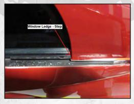
Peel the backing from the adhesive tape and place the louver over the quarter window. First, line up the bottom edge of the louver with the window ledge as shown.
