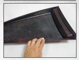
Wipe down the 5 tape ledges on the rear of the louver with the supplied alcohol pads, followed by the included 3M Adhesion Promoter pads.
