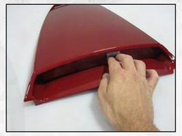
Use one of the supplied alcohol prep pads to thoroughly wipe down the area of the louver where the insert will be applied.
