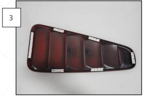
Place the supplied 3M Dual-Lock on the louvers' mounting points, then attach the mate to each of the six Dual-Lock strips that were just adhered to the louver.
