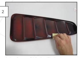
Using the supplied 3M Adhesion Promoter Pad, thoroughly wipe down the mounting points on the louver as well as the outside of the quarter window where the louvers will adhere. \*\*\*Only use one Adhesion Promoter Pad per side\*\*\*
