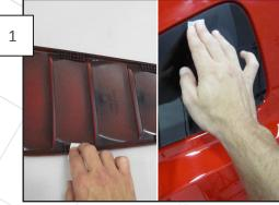
Using the supplied alcohol prep pad, wipe down the mounting points on the louver as well as the outside of the quarter window where the louvers will adhere. \*\*\*Only use one alcohol pad per side\*\*\*
