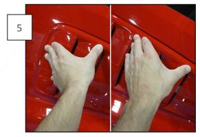
Once the louver is properly positioned around the quarter window, firmly press down around the entire edge of the louver to fully lock in the Dual-Lock. Repeat Steps 1-5 for opposite side louver to complete the installation. \*\*\*To clean, separate the 3M Dual-Lock by pulling up from one of the corners\*\*\*
