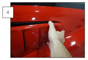
Peel the backing from the 3M Dual-Lock and place the louver lightly over the quarter window starting with the rear most portion as shown. Do not press down on the louver to fully seat the adhesive at this point.
