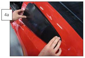
Starting from the rear, place the window cover over the glass. Keep forward pressure on the cover as you lay the front in place, this will ensure the part is seated properly over the glass.
