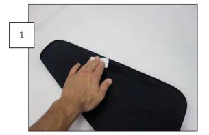
Use the provided alcohol pad to wipe down the back side of the window cover and the quarter window glass where the tape will adhere.
