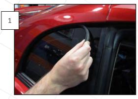
There is a small piece of rubber weatherstripping on some 99-04 cars that will have to be removed prior to installation. If it is present on your vehicle, simply start pulling the strip out as shown in the photo below until it comes completely out of the channel. \*\*\*Removing the rubber strip will not cause any issues, as the negative space will be taken up by the window cover and prevent any possible leaks\*\*\*
