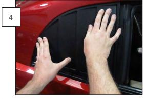
Place the cover on the window, aligning it first with the bottom rear corner and weatherstripping. Once the it is properly aligned, press down firmly around the outside edges to fully seat the adhesive. Repeat Steps 1-5 for the opposite side.
