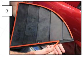
Peel the backing from the 3M Adhesive as shown below.
