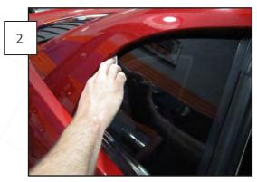
Using the supplied alcohol prep pads, thoroughly clean the outside edges of the quarter window where the adhesive will attach.
