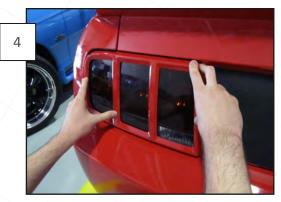
Starting with the upper inner corner, apply the trim to the tail light lens as shown below. Make sure there is proper clearance between the trim and decklid panel in the upper corner of the tail light.
