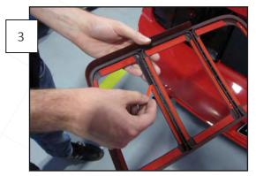
Peel the backing from the 3M Adhesive as shown.
