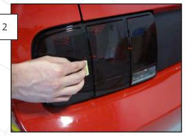
Apply the included 3M Adhesion Promoter to the same areas cleaned in Step 1. Only prep the very outside edges of the lenses where the adhesive will attach, there is no need to wipe down the entire lens.
