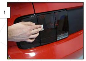
Using the supplied alcohol prep pads, thoroughly clean the outside edges of the three lenses where the adhesive will attach.
