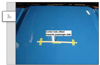
Once in the correct position, tape the template to the hood as shown. (*Make sure center hole is offset towards passenger side as seen above*)
