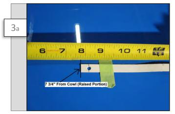
Measure 7 ¾" from the edge of the cowl (raised portion of hood) on either side to center the drill template.
