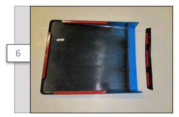
Apply the supplied adhesive tape to the areas wiped with Adhesion Promoter.
