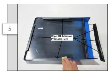
Lay the scoop upside down on something soft so as not to damage the finish. Wipe the supplied 3M Adhesion Promoter on the reverse side of the insert and the tabs of the scoop.
