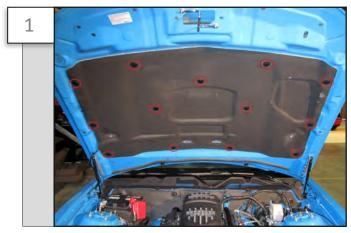
Using a trim removal tool or side cutters, carefully remove the 13 push pins securing the hood insulation pad and set it aside.
