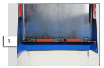
Install the 3 included U-Studs on the scoop insert.
