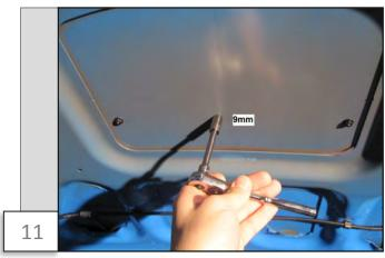
Once you are sure the scoop is centered, press down firmly around the edges and the front insert to fully seat the adhesive. Open the hood and install the nuts on the U-Studs. Tighten firmly with a 9mm socket.
