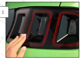
Use the supplied alcohol pads to thoroughly wipe down the areas where the adhesive tape from the tail light trim will contact the light.
