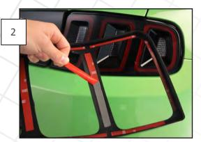
Peel the backing from the 3M tape as shown above.
