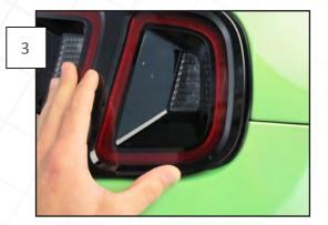
Beginning with the outside edge, carefully place the trim over the tail light, making sure to align the edges of the trim with the edges of the LED surrounds on the light. Do not press down at this point to fully seat the adhesive.
