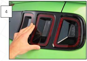
Once the trim is properly located, firmly press down to fully seat the adhesive tape.
