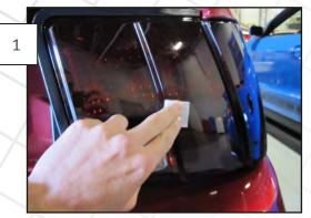
Open the trunk of the vehicle to allow for easier installation. Use the supplied alcohol pads to thoroughly wipe down the areas where the adhesive tape from the tail light trim will contact the light.
