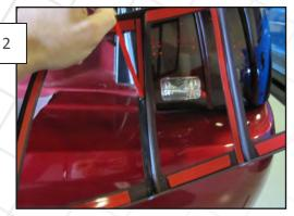
Peel the backing from the 3M tape as shown above.
