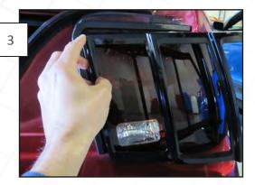
Beginning with the inside edge and working towards the outside, carefully place the trim over the tail light. Do not press down at this point to fully seat the adhesive.
