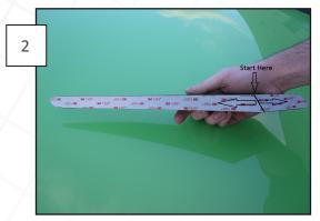
Starting from the rear transition edge of the splitter, install the provided 3M tape as shown.
