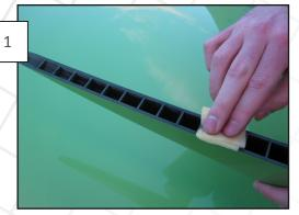
Using the supplied alcohol prep pads, thoroughly wipe down the back of the head light splitter and the center of the headlight lens where the splitter will attach. Once the alcohol has dried, repeat above steps using the included 3M Adhesion Promoter Pads.
