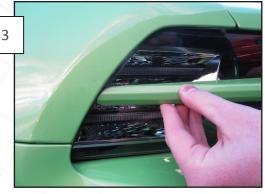
Remove the backing from the 3M tape and install the splitter onto the headlight.
