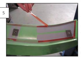
Place the four included foam pads over the threaded insert holes in the spoiler as shown. Peel the backing from the adhesive tape on the underside of the spoiler.
