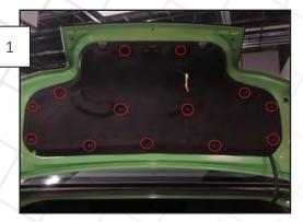
Using a trim removal tool or similar, remove the 13 plastic clips securing the trunk liner to the decklid and remove it from the vehicle.
