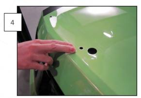
Once the decklid is clean and free of adhesive, wipe down the surface with the supplied alcohol pads as shown. Be sure to wipe all areas that the adhesive on the new spoiler will come in contact with.
