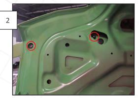
Remove the four 10mm nuts securing the factory spoiler to the trunk lid. \*\*\*Be sure to have someone holding the spoiler so it does not drop and hit the vehicle once the nuts are removed.\*\*\*
