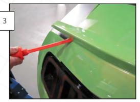
Close the lid and use a plastic chisel or similar tool that will not scratch your paint and remove the spoiler from the decklid. Once the spoiler is removed, use adhesive remover to clean up any residue left by the factory adhesive tape.
