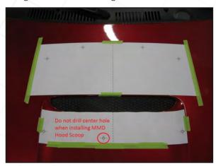
STEP 3b // The upper template is installed on the upper edge of the factory scoop, using the dotted center line as a guide (this dotted line should be matched with the dotted line on the lower template).
