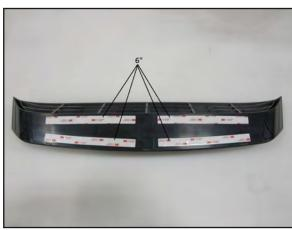
STEP 6b // Once attached to the insert, place the remaining 3 pieces of tape on the underside of the insert.
