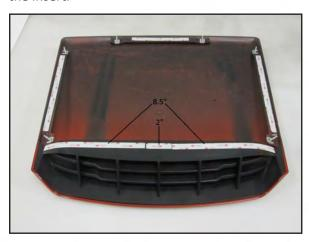
STEP 7 // Peel the backing from the adhesive tape and place the scoop on the hood aligning the rear studs first. Don't fully press down on the scoop until all studs are properly located and the scoop is in its desired location. Once it is properly aligned, move around the edges and firmly press down to fully seat the adhesive.
