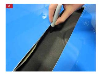
STEP 8: Test fit the hood liner and mark the opening and trim.
