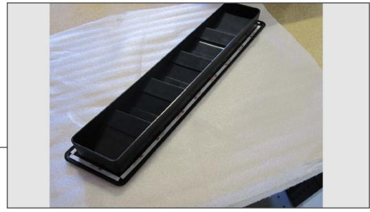
Lay the vents upside down and run the indented tape ledges with the supplied alcohol pads, followed by the supplied 3M Adhesion Promoter. Once dry, place the tape strips into the indented surfaces as shown. Be sure to put the tape as close to the outer edge of the indented surface
