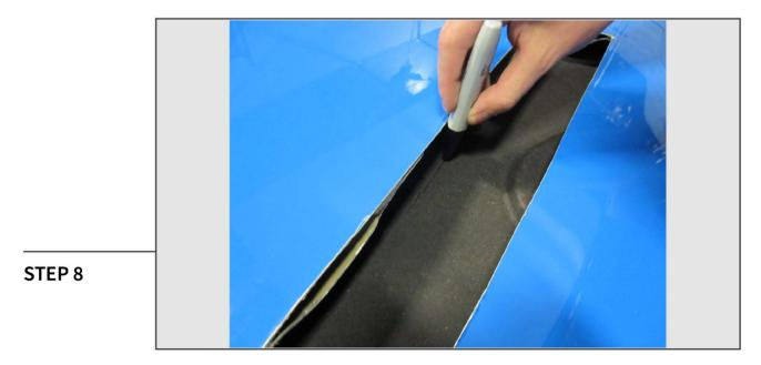
Remove the backing from the 3M tape on the top of the insert and install it into the scoop body. Place the front edge of the insert in first then firmly press down to fully seat the adhesive tape.
