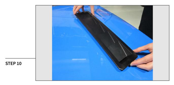
Remove the backing from the tape on the vents and lay them in the holes. Make any final adjustments necessary at this point before seating the tape. Once properly aligned & adjusted, press down firmly around all edges of the vents to fully seat the adhesive tape.
