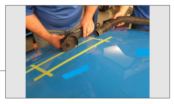
Lay some towels, newspaper, etc over the part of the hood that will not be cut to protect the paint. Using an angle grinder carefully cut out the areas that you masked off in Step 2. To avoid excess metal shavings, having someone follow with a Shop Vac is helpful.
