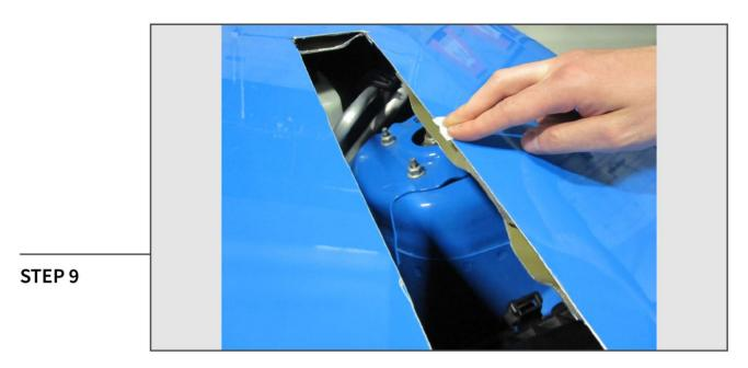
Thoroughly clean the edges of the holes using the supplied alcohol prep pads. Once dried, rub the edges with the supplied 3M Adhesion Promoter.
