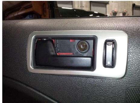
Step 4: Pull the inner door handle out and pop the inner cover out exposing the torx screw below.
