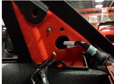
Step 3: Remove the 3 Bolts holding the old mirror in place.
