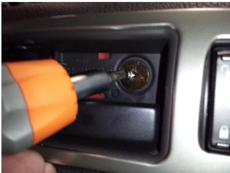
Step 8: Remove the T-30 torx screw behind the door pull and the door handle.
