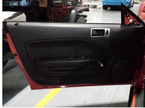
Step 9: Remove the 7mm screws located around the outer part of the door panel and pull the panel up and away from the door.
