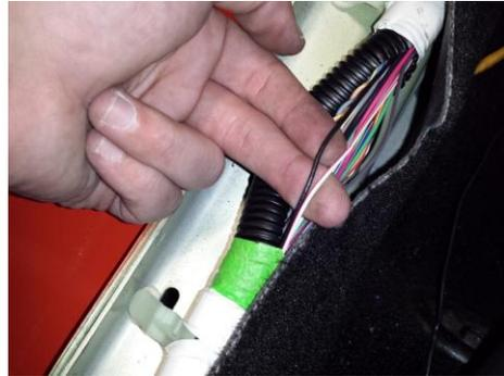
Step 4: Locate the wiring harness that runs down each door sill and expose the wires within.
