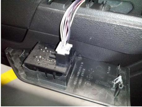
Step 6: Disconnect the wiring harness connected to the window switches and remove the 7mm screw behind it from the vehicle.
