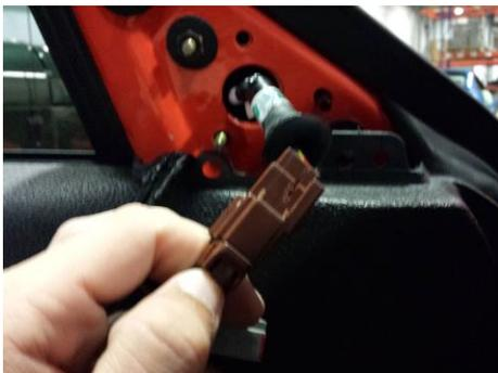
Step 2: Disconnect the harness connecting the door to the mirror control panel
