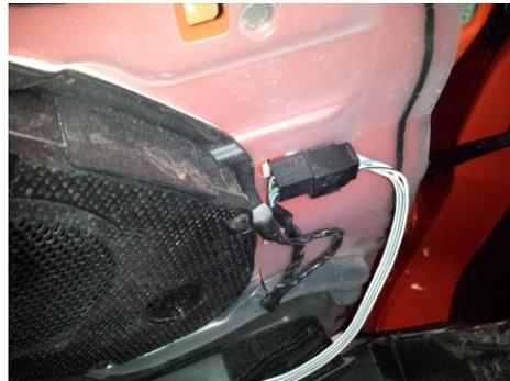
Step 10: Unplug all connectors holding the panel to the door leaving the door handle cable attached.
