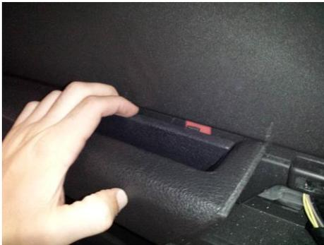
Step 7: Using your fingers or interior trim removal tools, pull the panel behind the door pull out and up to remove it from the vehicle.
