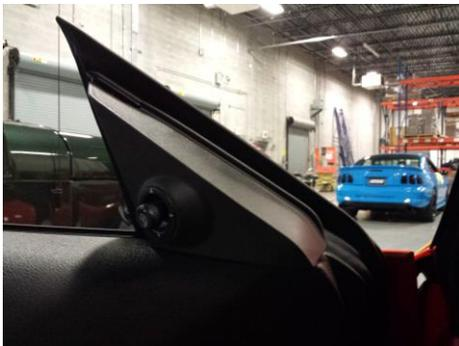
Step 1: Remove the driver's side mirror control panel by pulling away from the door
