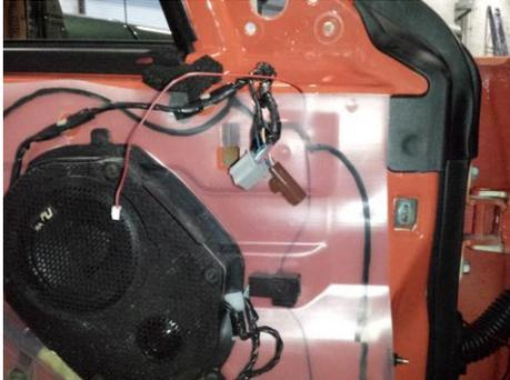
Step 1: Route the wire through the door panel and into the harness that passes through the vehicle.
