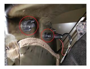
Pry back the trunk liner, and locate and remove the (2) taillight twist nuts.
