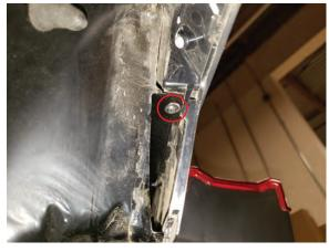
**Step 3**Using a Phillips head screw driver, locate and remove the screw securing the light to the trunk.
