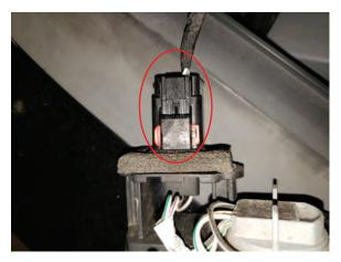
**Step 7**Carefully remove the outside taillights, and unplug the wiring connectors.
