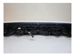
**Step 10**Twist, and unplug the factory wiring harness from the factory middle taillight assembly, and transfer to the new Raxiom middle taillight.
