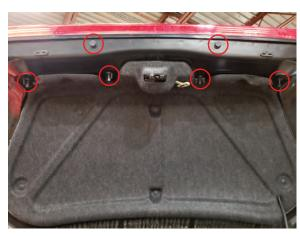
**Step 1**Begin by removing the (4) twist caps, and (2) bump stops located on the trunk.
