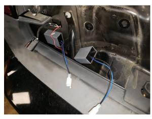
**Step 11**Install the (2) control boxes to the chassis of each side of the outside taillights. These control boxes are held in place by 3m tape. \*\*Note: Make sure these control boxes are not in the way of making contact with the taillights.
