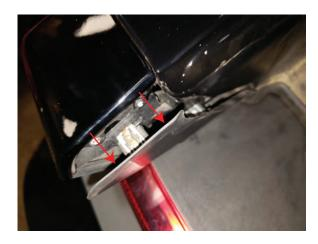
**Step 5**Using a panel removal tool, carefully pry the inside taillight trim piece covers away from the body of the vehicle.
