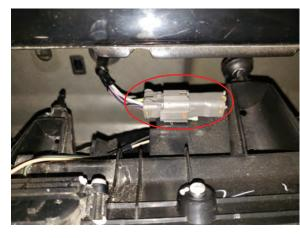
**Step 4**Carefully pry the light away from the trunk, and unplug the wiring harness connector.
