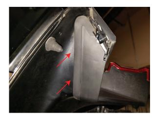
**Step 2**Using a panel removal tool, carefully pry the taillight cover off each side of the middle taillight.
