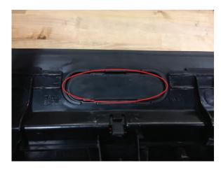
If your vehicle is equipped with the trunk release button, carefully cut out the middle section of the Raxiom taillight using a utility knife. Transfer the trunk release button from the factory light to the Raxiom light using the factory hardware.
