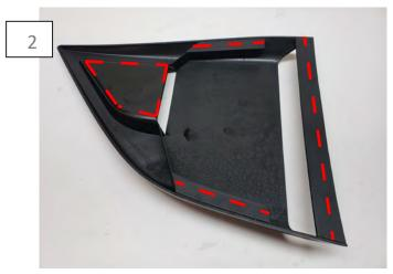
Apply the supplied 3M tape to the scoop as seen above. Test fit the insert on the scoop to familiarize yourself with how it fits.
