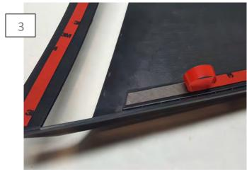
Remove the tape backing and install the scoop.
