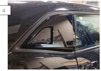
Apply firm even pressure to all taped surfaces to ensure proper adhesion.
