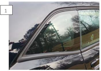
Wash the quarter window with soap and water. Allow the window and surrounding area to dry. \*\*Recommended: Wipe the window down with isopropyl alcohol to ensure the cleanest surface possible.
