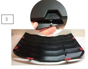
Remove the 8mm nuts for the mounting pads and install the mounting pads to rear window louver. Test fit the louver to the rear window prior to removing the tape backing. Familiarize yourself with how the lover fits. Center the louver side to side. Align the top edge with the top of the glass.
