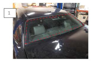
Begin by thoroughly cleaning the rear window glass using the supplied alcohol pad to ensure the glass is free of any and all road debris.
