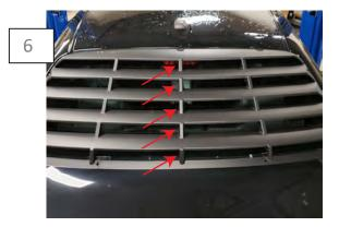
Install the supplied foam pads to prevent the louver from rattling against the window glass. It is recommended to install the foam with the louver already installed to ensure proper placement. Remove the tape back and install the foam so that the louver does not touch the glass.
