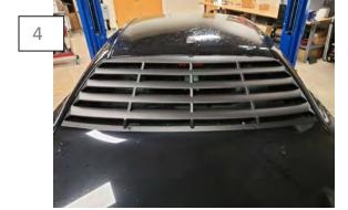
Once the rear window is clean/dry and free of contaminants, remove the red tape backing and set the louver on the window.
