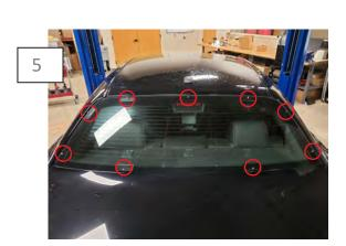
Remove the 8mm nuts and carefully remove the louver from the window. You want to make sure all of the mounting pads stick to the glass. Once the louver is removed, apply firm even pressure on all mounting pads to ensure proper adhesion to the window. Reinstall the window louver.
