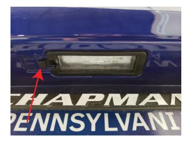
**Step 2:** Press and release the factory wiring connector from the factory light.
