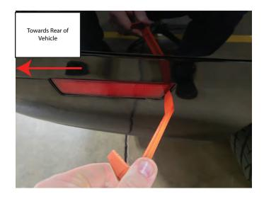
**Step 2:** Twist the socket counter-clockwise to remove from the factory light. Then remove the bulb from the socket.
