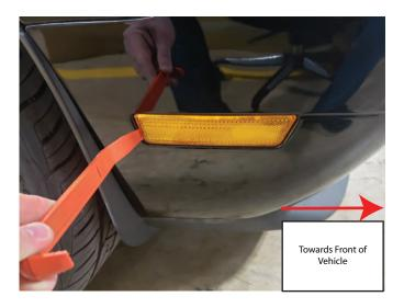
**Step 2:** Twist the socket counter-clockwise to remove from the factory light. Then remove the bulb from the socket.
