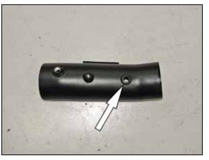
16. Using the provided grommet, Install the inlet air temperature sensor into the  $K\&N^{\otimes}$  intake tube,
