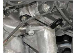
13. Install the tube mounting bracket (010088A) onto the cylinder head as shown. Be sure to place the provided spacer between the bracket and cylinder heads.
