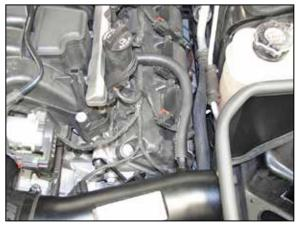
19. Install the provided crank case vent hose onto the fitting on the engine and then connect the open end to the vent on the  $K\&N^{\mbox{\tiny @}}$  intake tube,
