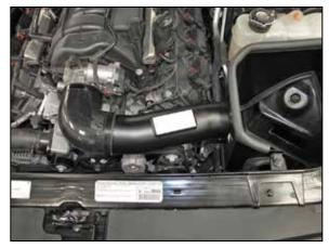
18. Install the K&N<sup>®</sup> intake tube into the silicone hose and align with the mounting bracket installed earlier. Secure with the provided hardware and hose clamp.
