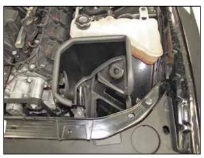
12. Install the heat shield into the vehicle and secure with the provided hardware. NOTE: Due to vehicle manufacturing tolerances the A/C lines of some vehicles may need to be repositioned slightly so they do not make contact with the heat shield or brackets.
