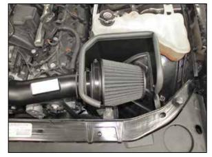
23. Install the filter assembly onto the  $K\&N^{\otimes}$  intake tube and secure with the provided hose clamp.
