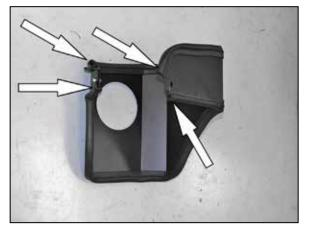
11. Install the two pieces of edge trim onto the heat shield as shown.
