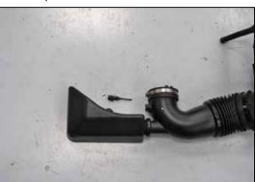
17. Install the appropriate 1/4npt fitting into the K&N<sup>®</sup> intake tube. The straight fitting is for 5.7L engines and the 90° fitting is for 6.0L. **NOTE: Plastic NPT fittings are easy to cross thread. Install the vent fitting "hand" tight, then turn it two complete turns with a wrench.**
