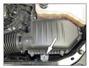
7. Remove the bolt which secures the air filter housing to the core support and then remove the complete air filter system from the vehicle. **NOTE: K&N Engineering, Inc., recommends that customers do not discard factory air intake.**
