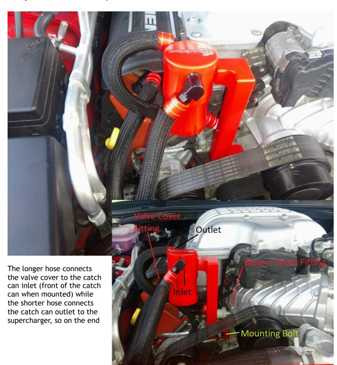
of the longer hose opposite the catch can, you will want to insert the black factory fitting and in the shorter hose, you want to install the white fitting from the factory hose assembly. In the image below, I have marked each of the key points of this install.
