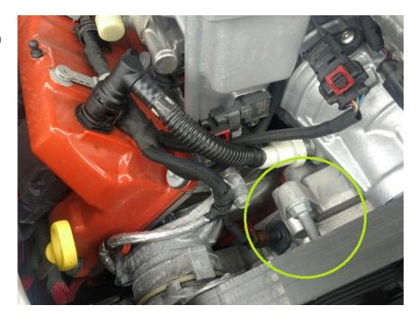
At this point, you are just about ready to install your American Brother Designs oil catch can, but first you need to remove the factory crankcase pressure hose fittings for use with the hoses that come with the kit. In reading around online, it seems that both of these fittings will pull out of the hose if you heat the hose up, but I am too impatient for that. The black fitting popped right out, but I couldn't get the white one out, so after a few seconds of
