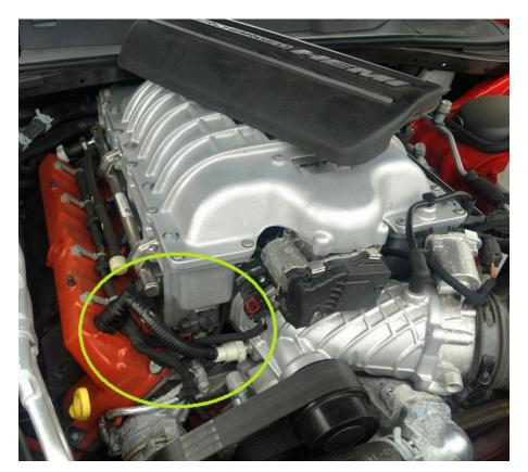
Step Two: Locate the crankcase pressure tube on the passenger's side of the engine. It is about 5 inches long and it runs from the front end of the valve cover to the lower area of the supercharger snout. It is circled in green in the image above.
