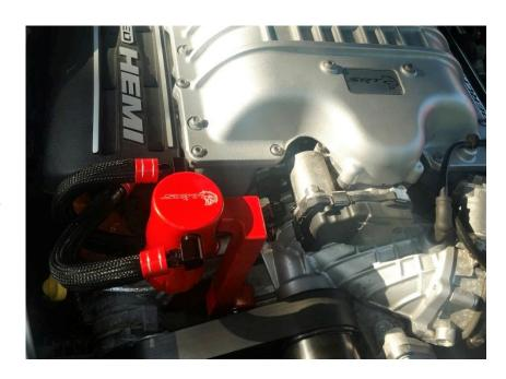
It should be noted that the hoses come longer than you will need, so you can trim them to a length that you like, but you can install the catch can with the longer hoses. I installed the can with the full-length hoses at first it worked just fine` without causing any interference elsewhere in the engine bay, but the engine bay looks much tidier with the hoses trimmed up as shown in the final image below.
