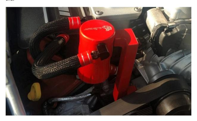
**Step Five:** Bolt the catch can in place with the included bolt and an Allen wrench, using the alignment pins in the bracket to position the assembly. Once that bracket is tightened down, plug in the black fitting to the valve cover, plug in the white fitting to the blower snout and that is it - the American Brother Designs catch can is installed and ready to begin keeping vaporized oil out of your induction system.
