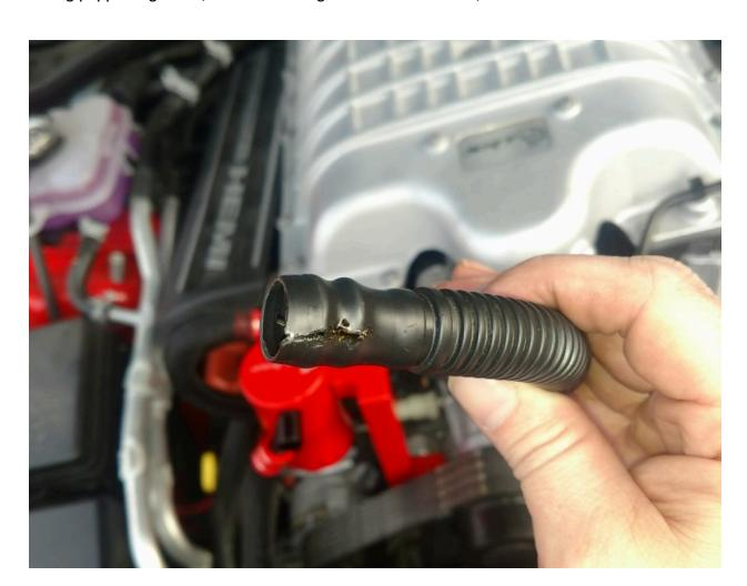
wrestling with it, I used a sharp knife to carefully cut the hose around the white fitting, as shown in the image below. With that done, you are ready to install the catch can.
