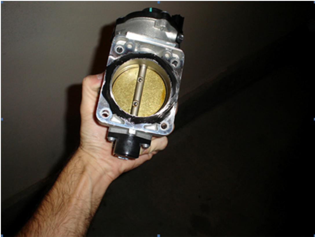
Figure 8: Throttle body with spacer attached and sealant applied
