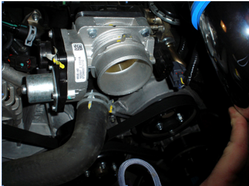
Figure 5: Cold Air Intake removed from the throttle body
