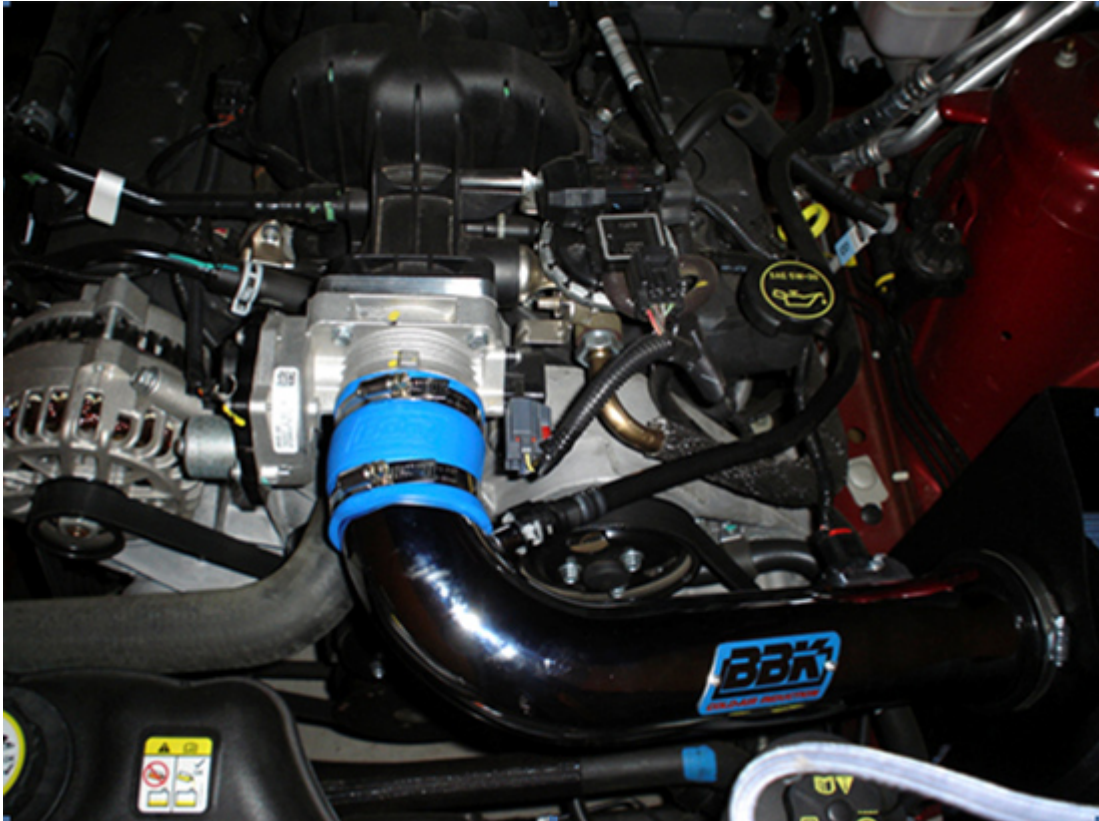
Figure 9: V6 Engine with throttle body and spacer attached. Cold Air Intake and power reattached
