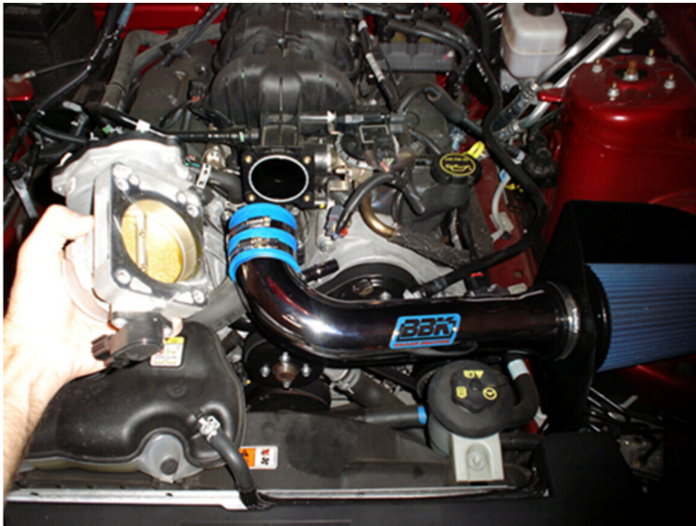
Figure 7: Removing the throttle body from the engine
