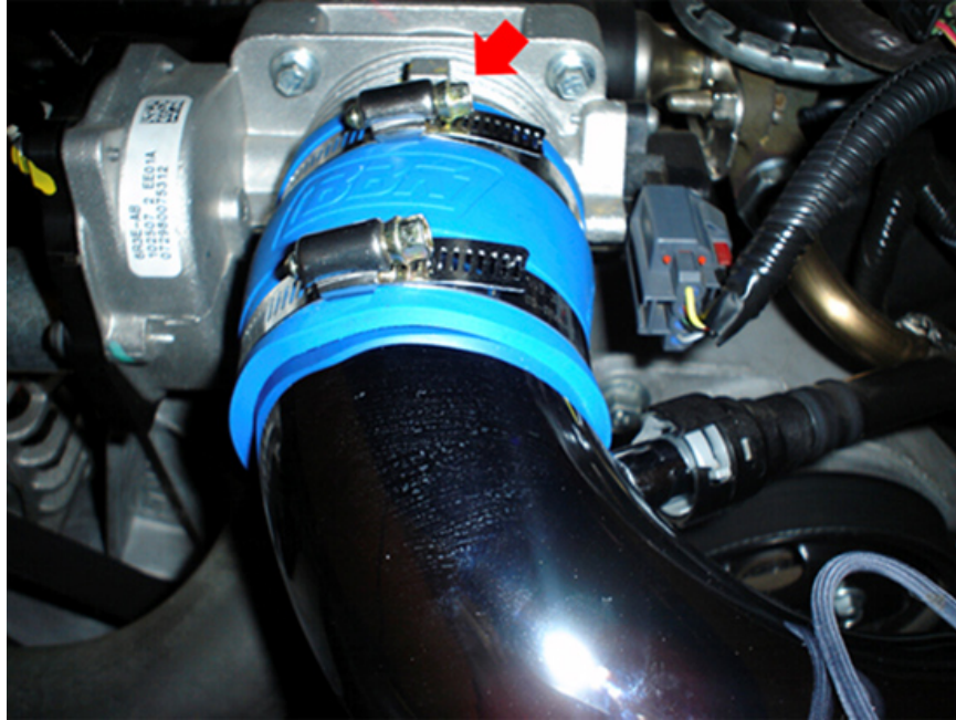
Figure 4: Loosen clamp from throttle body
