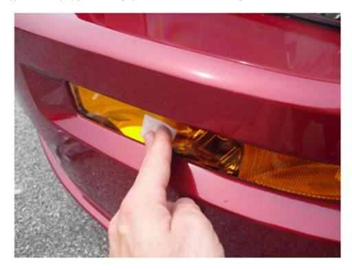
2. Peel backing from the adhesive tape and place cover over turn signal lens, making sure that the entire lens is covered. Once in proper position, firmly press down on cover to full seat the adhesive. Repeat instructions for opposite side cover to complete the installation.
