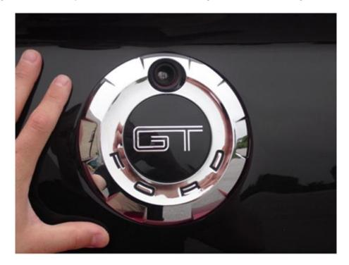
3. Once the panel is centered and the edges are covering all painted surfaces of the decklid, firmly press down on all areas of the panel to fully seat the adhesive.
