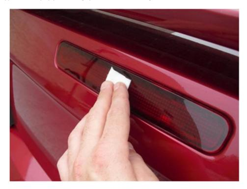
2. Peel backing from adhesive tape and place cover over the third brake light. When cover is properly aligned, firmly press down to fully seat the adhesive.
