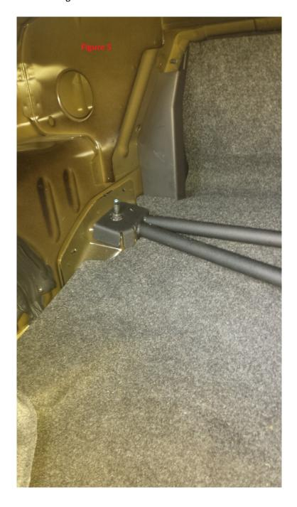
6. Install Flanged Nuts with rubber grommets back to the Studs as shown in Figure 6. ( Note, you may need to bend some of the fingers on the brace to allow it to sit right as shown in figure 7 )
