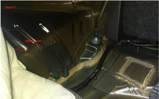
3. Use the 6mm wrench and adjustable wrench in Figure 4. On the driver side you will want to turn the nut towards the front of the care to loosen it. The 6mm wrench is used to keep the stud from turning.
