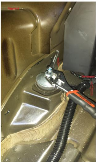
4. Perform the same operation with the 6mm and adjustable wrench on the passenger side. You will want to turn the adjustable wrench towards you and the 6mm wrench towards the front of the car. Remove both flanged nuts with rubber grommets and set aside
