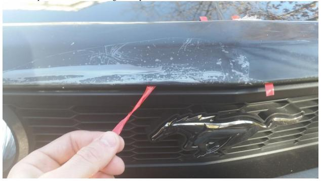
Step 7: If you are satisfied with the way the bottom tape seated, start removing the tape cover from the top strips one at a time, working from the center to the end.
