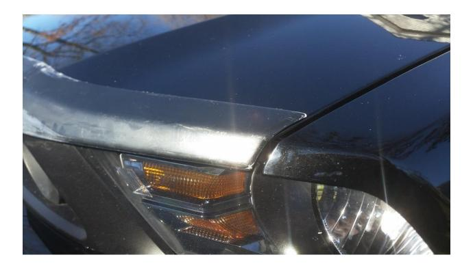
Step 5: When you are satisfied with the alignment, push down in the center, seating the tape that you exposed earlier.
