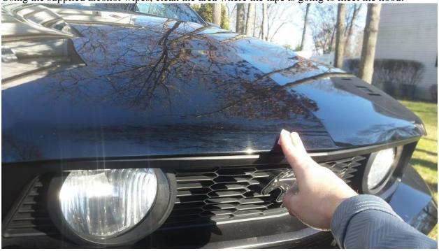
Step 3: Peel a small section of the tape cover away from the inside sections, making tabs that stick past the outside of the hood deflector so you can grab them later.
