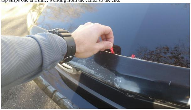
Step 8: Remove the plastic cover from the hood deflector. Re-check to make sure you are happy with the alignment.
