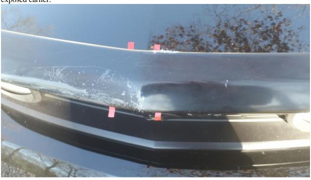
Step 6: Starting with a bottom strips, one at a time start peeling the tape cover away, pressing down on the hood deflector as you go to seat the tape. Work from the center out towards the ends. Make sure to keep the hood deflector aligned as you do this.
