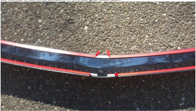
Step 4: Carefully align the hood deflector on the hood, making sure both ends are even with the hood. It helps if you have a second person to hold the hood deflector in place.
