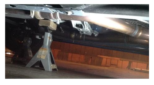
3. Before loosening any bolts, you can add reference marks on the body and cross member to help you line up the cross member during reinstallation. With the car and transmission safely supported, remove the four outer bolts holding the transmission cross member to the car with an 18mm socket and ratchet.
