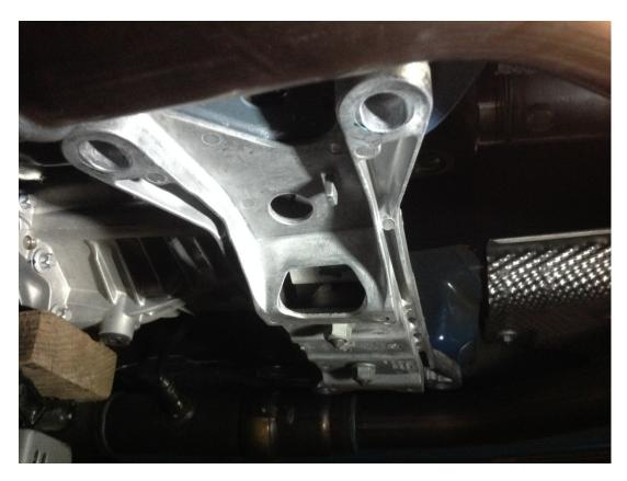
4. Next, remove the two nuts holding the cross member to the transmission mount using a 15mm socket and ratchet. These two nuts are the only thing holding the cross member on the car. Safely remove the cross member to expose the transmission mount.
