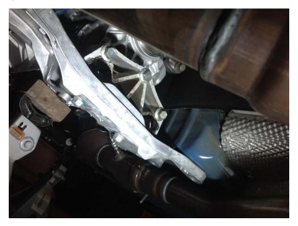
7. Replace the four bolts to secure the cross member to the car. Tighten them hand tight first, then tighten them with the 18mm socket and ratchet. Tighten the four outer bolts first, then the two nuts.
