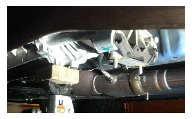
5. My insert did not come with grease or instructions to use grease, but I put a little on the ends of the mount to facilitate placement of the transmission mount insert. Simply slide the insert into the transmission mount from the front of the car towards the back and push it all the way into place.
