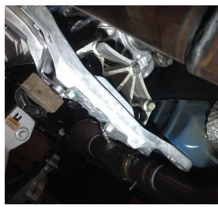
7. Replace the four bolts to secure the cross member to the car. Tighten them hand tight first, then tighten them with the 18mm socket and ratchet. Tighten the four outer bolts first, then the two nuts.
