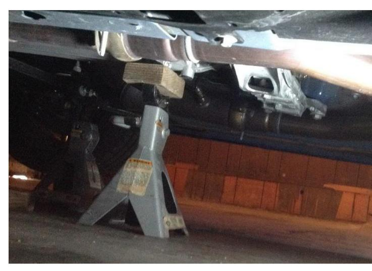
3. Before loosening any bolts, you can add reference marks on the body and cross member to help you line up the cross member during reinstallation. With the car and transmission safely supported, remove the four outer bolts holding the transmission cross member to the car with an 18mm socket and ratchet.
