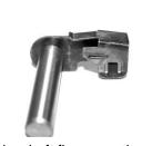
9. Remove the two nuts that attach the rear shifter mount to the chassis just above the driveshaft flange on the transmission. Remove the shifter from the car.
