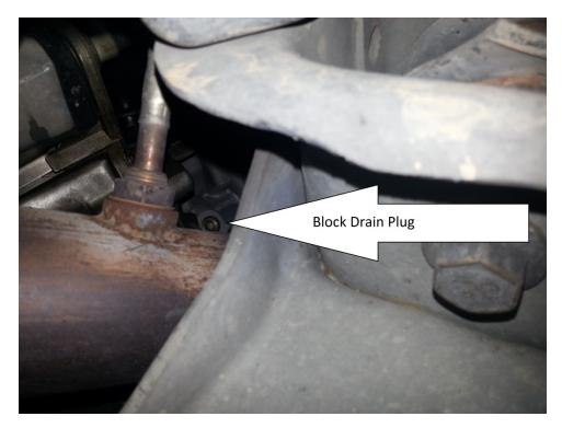
4. Once the block drain plug is out and it has finished draining, it is a good time to flush the system to remove any sediments. Remove the lower radiator hose using a large pair of pliers. Now remove the crossover tube plug and attach water hose there. Hold/Flush the water hose there until the water from the lower radiator hose and block drain plug run clear. Reinstall the block drain plug.
