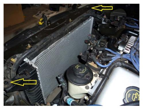
10. Shove a rag in the bottom radiator hose connection to prevent coolant from leaking out when lifting the radiator.
