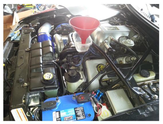
21. Start car, place heater on max and let it warm up until the thermostat opens and coolant cycles. The funnel will bubble indicating air is being released, if the coolant drops below the funnel, add some slowly until you have some remaining in the funnel. Do not let it run so long that the coolant begins to rise in the funnel.
