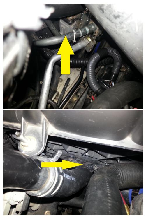
8. Remove the two bolts that hold on the fan shroud to the radiator about half way down each side of the shroud. Once bolts are removed, pull straight up to remove the fan/shroud assembly.
