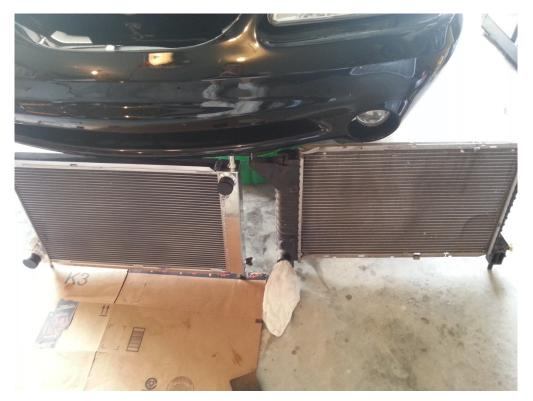
13. Gently slide new radiator in place being careful not to bend any fins. Get it close to seated and then get under the car and guide it in to place. There is minimal clearance between the new radiator and the ABS unit on the passenger side. I slid a piece of foam in between them just in case they rub. If there is not enough clearance, you could notch the abs unit bracket holes and slide it over a bit, or modify the bottom radiator mount.
