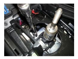
7. Gently pull the shifter out of the vehicle through the passenger compartment.
