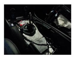
Remove the rubber insulation and rubber boot from the factory shifter.
