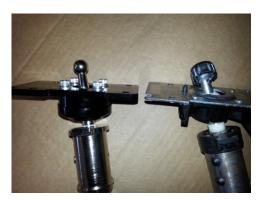
Install the new shifter into the vehicle by sliding it back onto the shifter assembly and bolding it down using the factory hardware.
