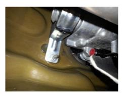
6. With the shifter assembly now lowered, remove the (4) 10mm bolts holding the shifter itself to the assembly.
