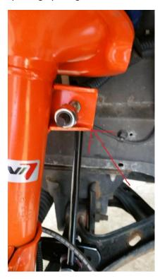
6. Install the bottom end link nut onto the end link using a 19mm wrench and 8mm wrench.
