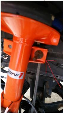
3. Next, remove the bottom end link nut from the shock mount using an 18mm socket. Same as the top nut, you will probably need to use an 8mm wrench or adjustable wrench on the back of the end link to keep the end link from spinning. Remove the end link and put the end links and nuts aside – the parts will not be reused.
