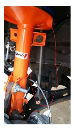
2. Remove the top end link nut from the sway bar using an 18mm socket. You will probably need to use an 8mm wrench or adjustable wrench on the back of the end link to keep the end link from spinning. If the end link does not require the 8mm wrench to keep it from spinning freely, it's probably seized.
