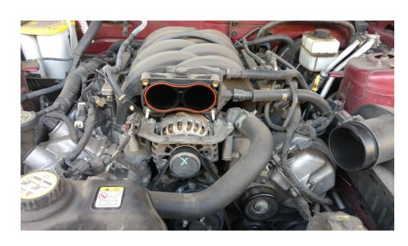
You can loosen the other side of the air intake hose and remove it completely. Otherwise just work around it.
