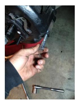
Step 2: With the 17mm socket tighten both bolts until snug followed by another 1/8 turn.
