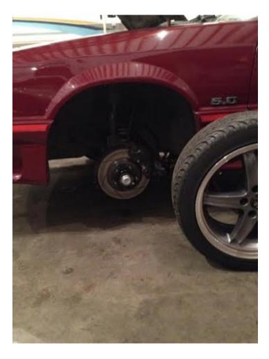
Step 4: With the ratchet and lug socket, using either 13/16 or 6 spline depending on lug nuts, remove the 4 or 5 lug nuts holding your wheel on and then pull the wheel off the hub.
