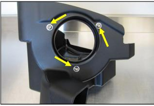
6. Install the filter adapter (#8) using three 1/4-20 button head bolts (#10), and flat washers (#11) into the Airaid Cool Air Box as shown.
