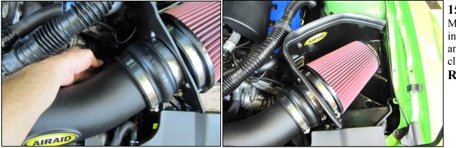
13. Reconnect the Mass Air Flow sensor, which is now 14. Install the Weather Strip onto the Cool Air Box with located in the lower back side of the intake. Slide the locking tab back into the connector.
