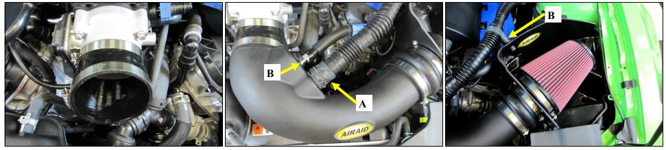
10. Install the Silicone Reducer (#6) and Hose clamps onto the throttle body. Place the #56 clamp (#15) on the Throttle body side of the reducer, and the #64 clamp (#14) on to the tube side.
