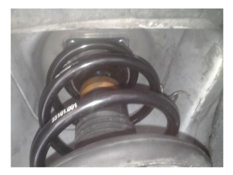
10. Reassembly is the reverse of disassembly. Reinstall the bolts that hold the bottom of the strut to the spindle. These should be tightened to 148 lb. ft. Reattach the sway bar end link to the strut and torque the nut to 85 lb. ft. Reattach the brake line bracket bolt and torque to 15 lb. ft. Attach the wheel speed sensor wire retaining clip by pushing it into the correct hole in the strut. The wheel can be reinstalled at this point. Tighten the lugs in a crisscross pattern.
