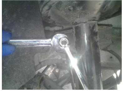
4. Remove the 2 strut to spindle nuts and bolts using a 15 mm socket and an 18 mm wrench on one bolt and an 18 mm socket and a 21 mm wrench on the other bolt. Once the hardware is removed pull the top of the spindle away from the strut so that the bottom of the strut swings freely.
