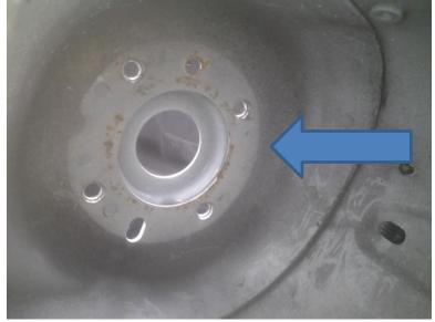
6. If necessary, using sand paper, remove any burrs or rough spots from the strut tower where the BBK plates will be located.
