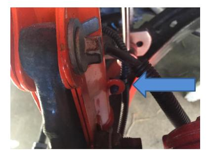
3. Unbolt the stabilizer bar link nut from the strut using a 19 mm wrench to loosen the nut while stopping the link stud from spinning with an 8 mm wrench. Once the nut is removed, push the stabilizer bar link through the mounting hole in the strut.
