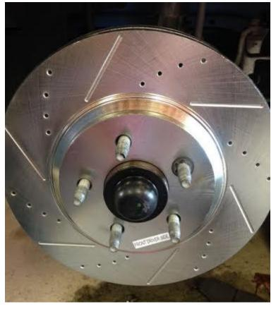
15. Once new rotor is in place, install new metal spring clips on the fixed part of the caliper and reinstall this portion of the caliper by tightening the two bolts using a ratchet and 15mm socket.
