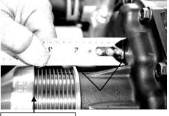
Align pulley tool here
