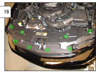
10-12 CARS: Remove the (8) push pins, holding the radiator cover to the car, by prying them with a small screwdriver. Remove the radiator cover, by pulling up on the back of it and pulling it toward the back of the car.
