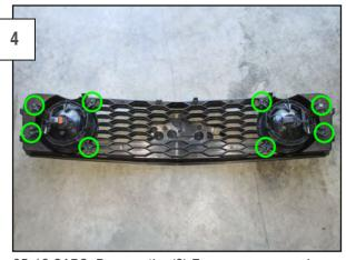
05-12 CARS: Remove the (8) 7mm screws securing the fog light mounts to the grill. (05-09 grill pictured, 10-12 looks different, but mounts are similar.)
