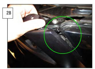
10-12 CARS: Press in on the grill tab, until the lip securing grill into the front bumper is released. Move on to the lower tab, then over to the opposite side. There are tabs along the bottom of the bumper that will come loose with some force. Be careful, to keep from breaking the tabs or the bumper.
