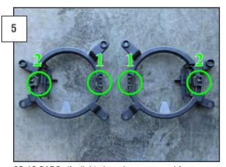
05-12 CARS: (foglights have been removed for illustration purposes) Be sure to mentally record how the fog lights are mounted with the vent on the top side. Pull the inner mount tab away from the fog lights. When it is released, pull the inner side of the fog light away from the mount and the outer will follow. Reinstall the lights in the reverse order, insert the outside of the mount into the light, then lower the inner side of the light to the mount until it snaps in.
