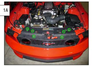
05-09 CARS: Remove the (6) push pins, holding the radiator cover to the car. Remove the radiator cover, by pulling up on the back of it and pulling it toward the back of the car.
