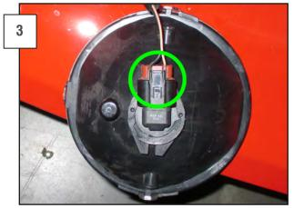
05-12 CARS: Press down on the electrical connector to release the fog light harness from the fog lights.
