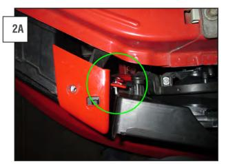
05-09 CARS: Press in on the grill tab, until the lip securing grill into the front bumper is released. Move on to the lower tab, then over to the opposite side. There are tabs along the bottom of the bumper that will come loose with some force. Be careful, to keep from breaking the tabs or the bumper.
