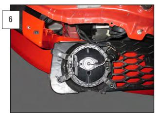
Reinstall the light mounts. Plug the vehicle harness into the back of the lights and push the grill back into the car, making sure the wires aren't near the radiator or other sharp/hot parts. Reattach the negative battery cable and make sure the lights are working. There is a screw on the back side of the fog lights that can be turned to adjust the beam up or down.
