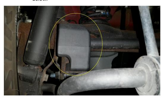
3. Remove 18 millimeter panhard bolt on driver side circled in the picture below.
