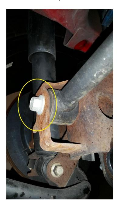
4. Loosen the panhard support bolt on passenger side circled in the picture below. Do not remove completely as it is unnecessary.
