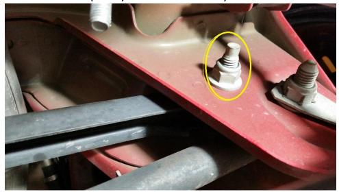
5. Carefully remove the 18 millimeter passenger side panhard bolt circled in the picture below. At this point the panhard bar will swing free from the bracket.
