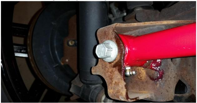
9. Push panhard bar up to align it into the passenger side mount pictured below. It may be necessary to use a tapered punch to align holes in order to slide the bolt through.
