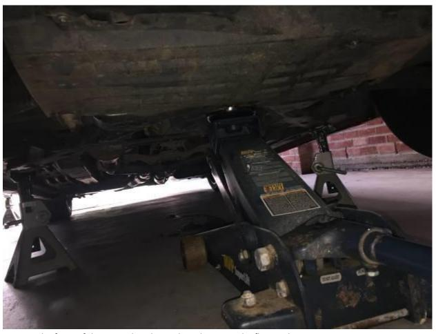
2. Support the front of the car with jack stands and remove the floor jack
