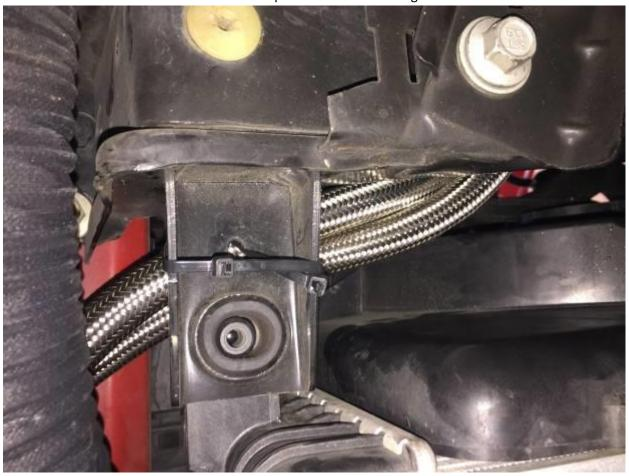
13. Connect braided oil line hose to fittings at sandwich plate, torque to 15-25 ft/lbs (do not exceed 35 ft/lbs) with -10AN wrench or 1" open end wrench
