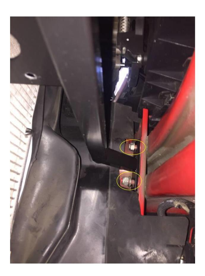
7. Attach the oil cooler to the bracket (11mm wrench) and then attach the braided stainless steel oil lines to the inlet and outlet fittings on the oil cooler. The longer oil line goes to the passenger side connection and the shorter line to the driver's side. Tighten -10AN fittings 15-25 ft/lbs, do not exceed 35 ft/lbs
