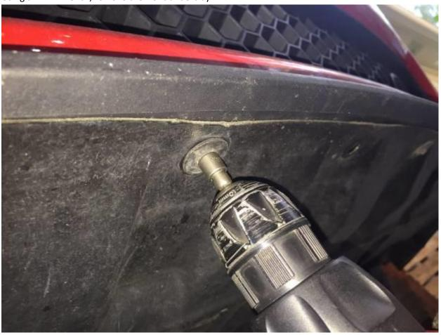
4. Using an 8mm wrench remove the rear engine undertray
