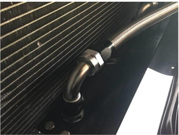
8. Route oil lines over the driver's side bumper support and secure to mounting bracket with cable tie
