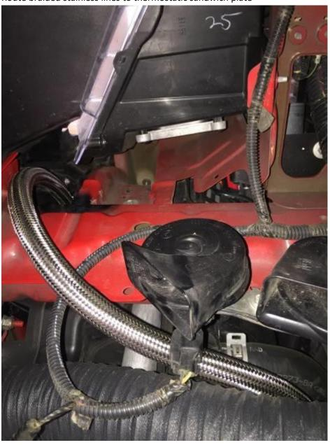
12. Route lines under lower radiator hose and above front swaybar. Use cable ties to secure braided hoses to lower radiator bracket – this will keep the lines from rubbing lower radiator hose
