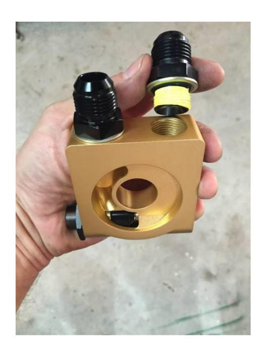
10. Remove oil filter, install sandwich plate with O-ring toward oil filter housing (-10AN wrench or 1" socket), install sandwich plate fitting and torque to 15-25 ft/lbs, do not exceed 35 ft/lbs.
