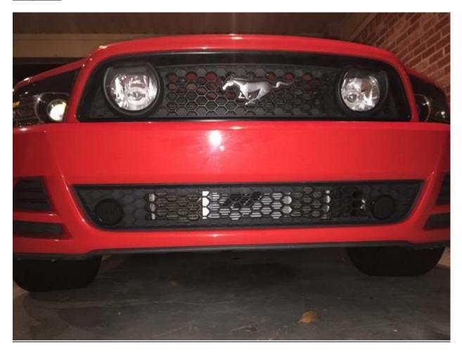
Congratulations, you have successfully installed the Mishimoto Direct Fit Oil Cooler! This oil cooler will reduce oil temperature up to 35°F, which is very important when running the car at high loads in hot temperatures such as High Performance Driver's Education track days during the summer.
