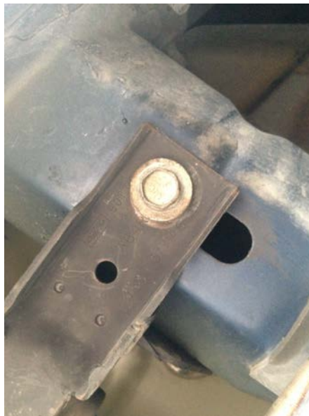
Figure 8: Rear Muffler Hanger Mount Bolt (Passenger Side Shown)
