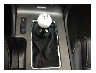
Then thread the shift knob on until it stops. Back the shift knob off so that the shift pattern is aligned properly. Then turn the retainer counter clockwise until it locks against the shift knob.
