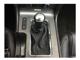
Remove the factory shift knob by rotating it counter clockwise. The shift boot is held onto the shift knob with tension, gently pull the off the factory shift knob
