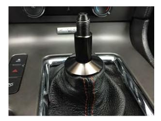
Install the supplied shift boot retainer. Thread the retainer on as far as it will go. Pull the shift boot onto the groove of the retainer.
